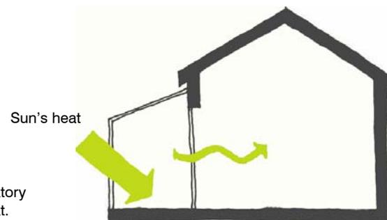
Diagram to show how a conservatory provides warmth by radiating heat.
